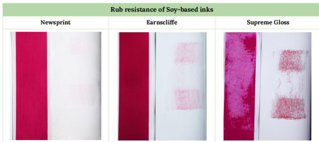
Figure 4. The ink rub resistance of the vegetables-based ink on the surfaces
