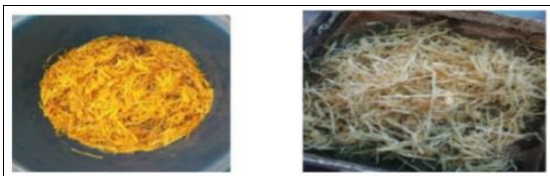
Figure 5. Bagasse fibre after treated in solution after 1 hour (a) 5% NaOH treated, (b) 5% HCL treated [10].
